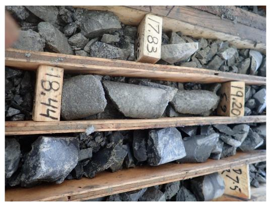
Figure 1. Quartz/feldspar porphyry with coarse disseminated arsenopyrite (18.44-19.20m).
