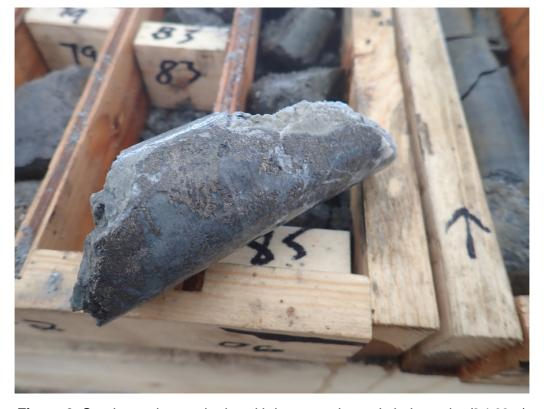
Figure 3. Semi-massive pyrrhotite with lesser pyrite and chalcopyrite (24.69m).
