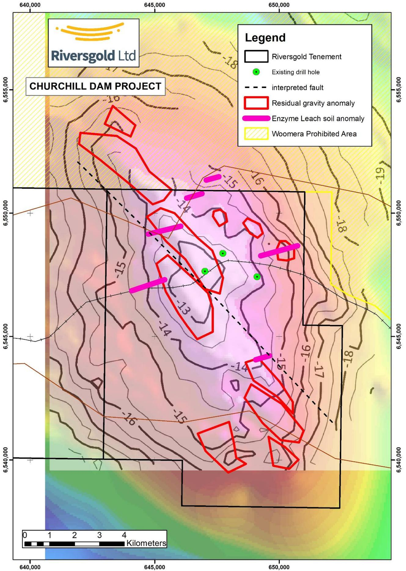
**Figure 2.** Churchill Dam Bouguer gravity anomaly with residual gravity and partial leach soil anomalies.
