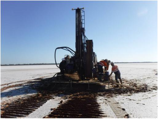
Figure 1. Aircore rig on Lake Yindarlgooda.
