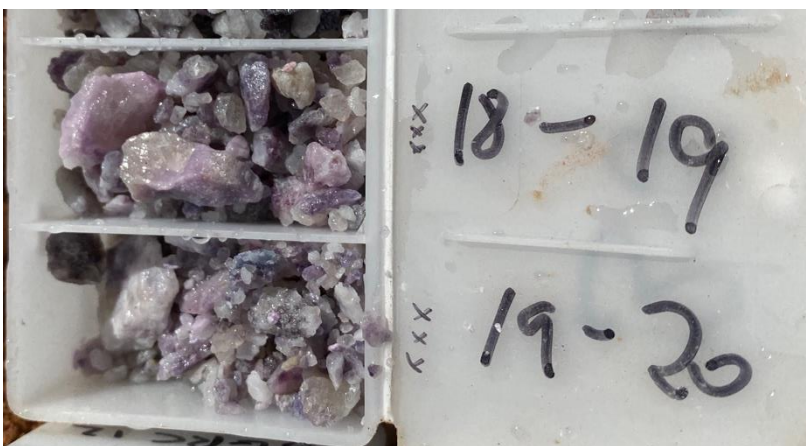
Figure 4: TMBRC003 from 18.0m to 20.0m interval within 13.0m pegmatite intercept in natural light showing lepidolite and spodumene mineralisation.
