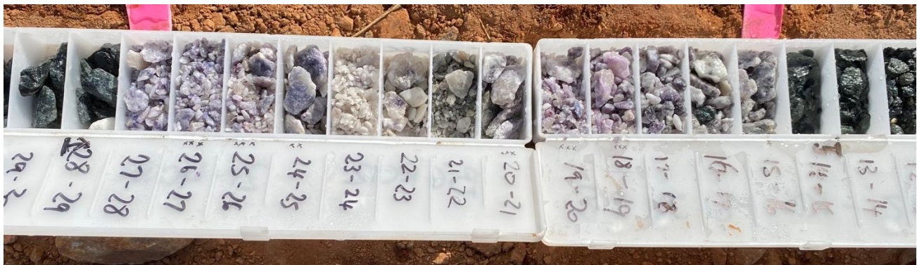
Figure 6: Chip tray for TMBRC003, showing interval 15.0m to 29.0 m
