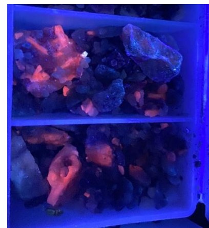
Figure 5: TMBRC003 from 18.0m to 20.0m under UV light showing spodumene in pink.
