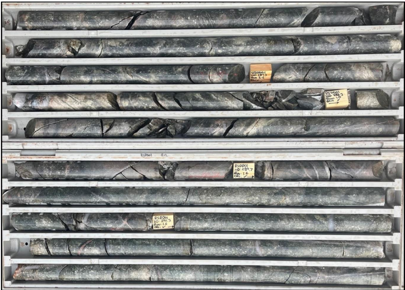
Figure 2: Northern Zone diamond drill hole RSDD001 (280m – 294m) wide zones of silica, albite and pyrite alteration
