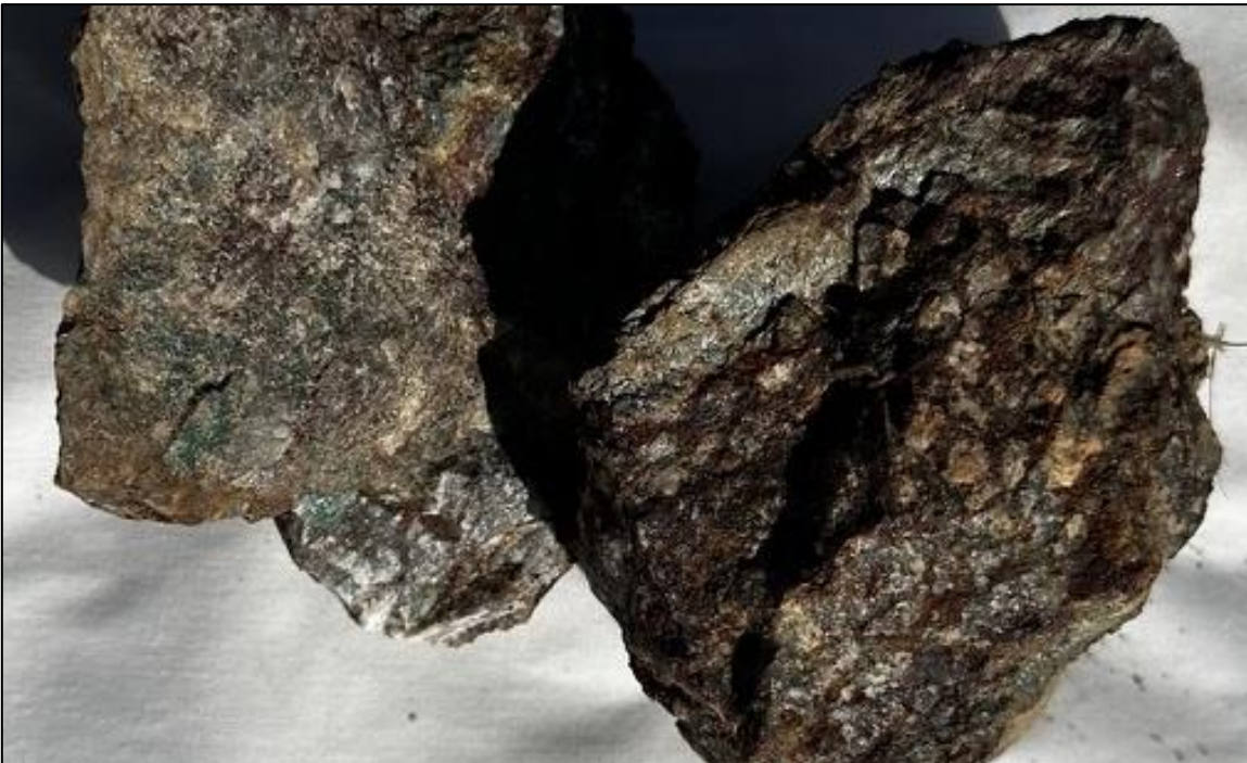
Figure 15: Lone Star Prospect sample TEM15 that assayed 4.11% Cu and 82.2 - 101 g/t Au (101 g/t Au = 3.2 Oz/t Au) 16
